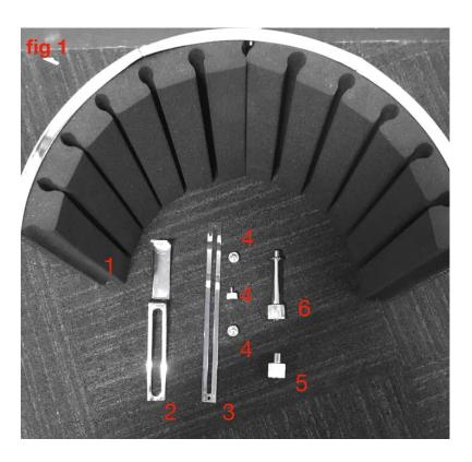
Attach 3 onto back of screen (1) use 4 to screw in place. As seen in fig 2
